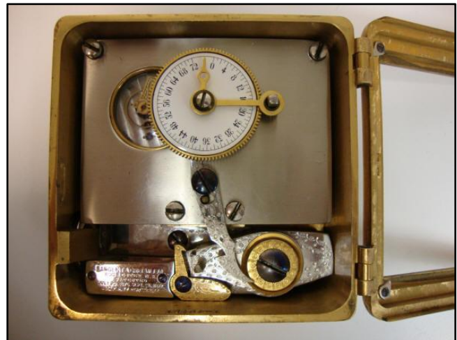
A Model No. 4 Corliss retrofit is shown with a Banker's Dustproof movement on the left and a Mosler movement on the right. Both examples were likely produced by Mosler Safe Company following its acquisition of Corliss Safe Company.
