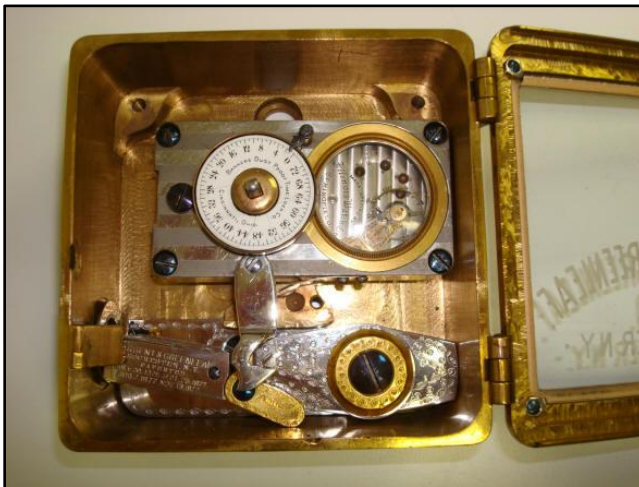
A Model No. 4 Corliss retrofit is shown with a Banker's Dustproof movement on the left and a Mosler movement on the right. Both examples were likely produced by Mosler Safe Company following its acquisition of Corliss Safe Company.
