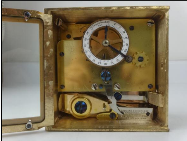
S&G Model 4 original, left, made exclusively for Corliss Safe Co. Retrofit likely by Andy Kotas, right.
