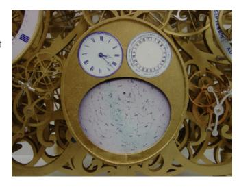
Sidereal time - (left dial, will be skeletonized), also known as 'star time'. During the course of one day, the earth has moved a short distance along its orbit around the sun, and so must rotate a small extra angular distance before the sun reaches its highest point. The stars, however, are so far away that the earth's movement along its
