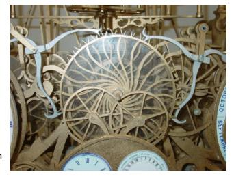
Since the period of the pendulums is four seconds, the main clock dial's second hand will move every two seconds. The remontoire are driven by a differential connected to the rest of the going train.
